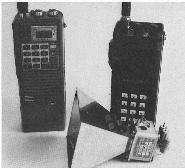
Fig. 1-8. A view of the future of Amateur Radio communications? A 10-GHz Gunnplexer and 2-meter hand-held transceivers combine to expand the horizons.
