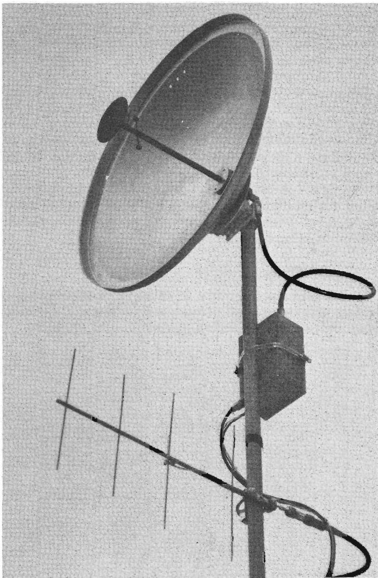
Fig. 4-5. A portable repeater system using 434-MHz input and 1277-MHz ATV transmitter. This system was used for coverage of the Pasadena Rose Parade.
