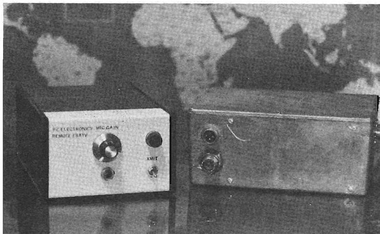
Fig. 4-2. A 1253- or 1277-MHz ATV transmitter system designed by W6ORG. The transmitter is in the weatherproof housing at the right, designed to be mounted at the antenna. The control box is at the left.
