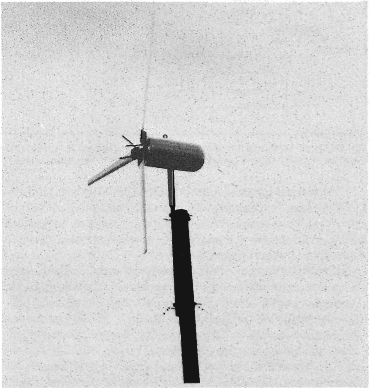
Fig. 8-5. A modern, 1500-watt, continuous-duty wind-powered generator provided by Windpower Corp. of Livonia, Michigan. The unit charges a bank of 12-volt batteries located at ground level.
