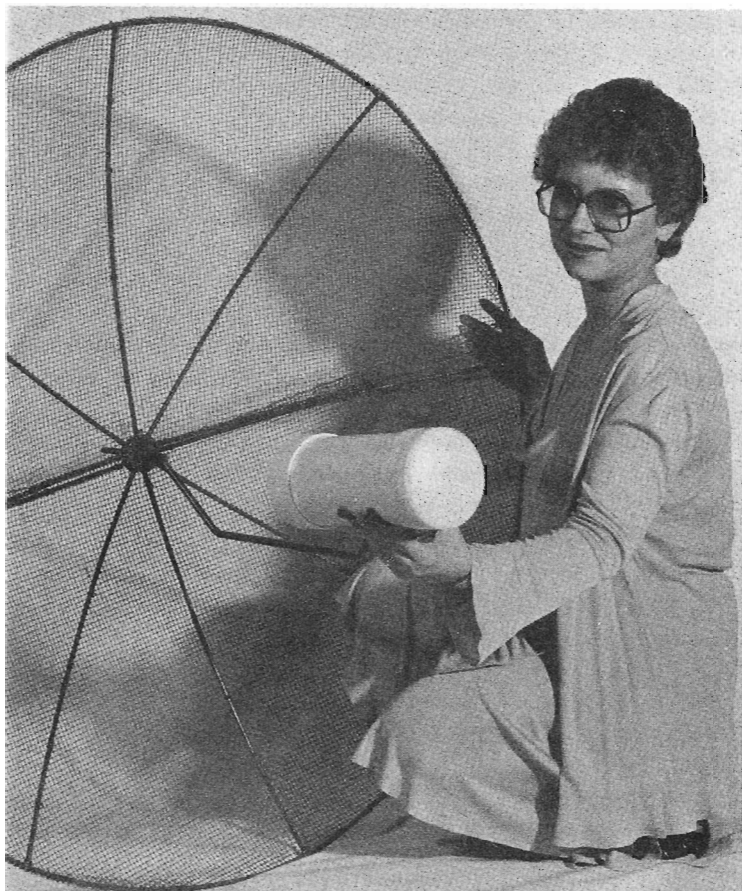
Fig. 9-1. This 4-foot parabolic dish antenna, demonstrated by Deborah Franklin, provides quality performance and high gain at 2.3 GHz.
